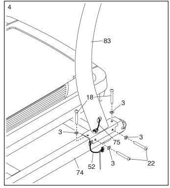
5. Connect the Base Wire (52) to the Upright Wire (75). IMPORTANT: The wire connectors should slide together easily and snap into place with an audible click. If they do not, turn one connector and try again. You must connect the wires properly for your incline trainer to function properly.
