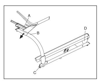
Carefully roll the incline trainer on the wheels to the desired location, and then lower it to the level position. CAUTION: To reduce the risk of injury, use extreme caution while moving the incline trainer. Do not attempt to move the incline trainer over uneven surfaces.
