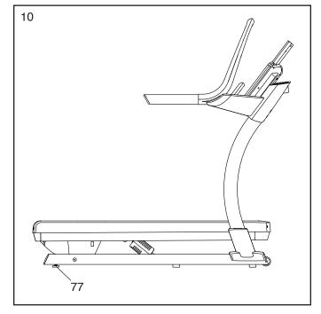
10. Make sure that all parts are properly tightened before you use the incline trainer. Keep the included hex keys in a secure place. One of the hex keys is used to adjust the walking belt (see pages 27 and 28). To protect the floor or carpet from damage, place a mat under the incline trainer. To avoid damage to the console, keep the incline trainer out of direct sunlight.
