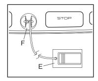
for the console to be ready for use. IMPORTANT: In an emergency, the key can be pulled from the console, causing the walking belt to slow to a stop. Test the clip by carefully taking a few steps backward; if the key is not pulled from the console, adjust the position of the clip.
