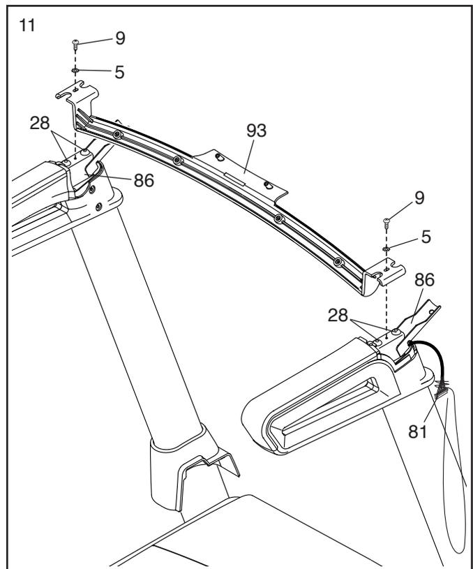
12. With the help of a second person, hold the console assembly (J) near the Handrails (86) (only one side is shown).
