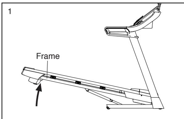
2. Raise the frame until the storage latch locks in the storage position. **CAUTION: Make sure that the storage latch locks.**
