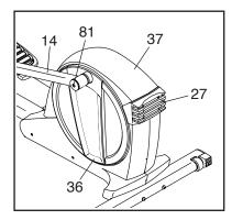
shown) from the Large Storage Foot (27), and remove the Large Storage Foot. Remove the two M4 x 16mm Screws (not shown) from the Top Shield (37), and then use a standard screwdriver to pry the Top Shield upward off the elliptical. Then, pry the left Pedal Disc (36) off the elliptical.
