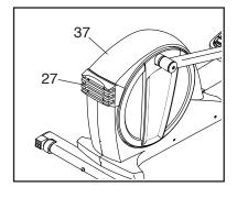
shown) from the Top Shield (37), and use a standard screwdriver to pry the Top Shield upward off the elliptical. Then, look into the access opening and locate the Reed Switch (58). Rotate the Pulley (66) until a Magnet (41) is aligned with the Reed Switch.
