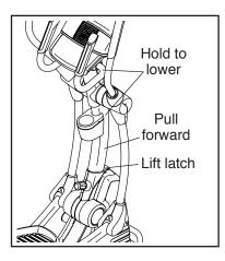
Next, hold the handle on the front stabilizer and lift the elliptical until it will roll on the wheels (not shown) on the rear stabilizer. Then, carefully move the elliptical to the desired location, and lower it to the floor.
