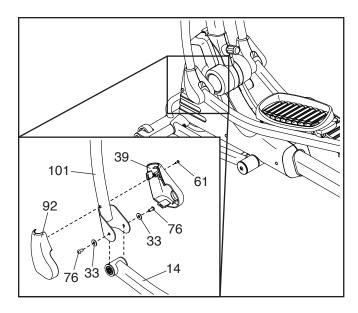
Then, remove the two M8 x 16mm Hex Screws (76) and the two M8 Washers (33) from the Left Upper Body Leg (101) and the Left Pedal Arm (14).
