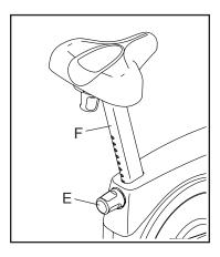
is engaged in one of the adjustment holes in the seat post. Then, turn the knob clockwise to tighten it.
