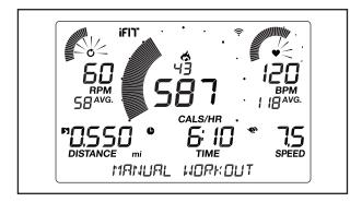
**Calories (flame icon)**—When the manual mode is selected, this display will show the approximate number of calories you have burned. When an
