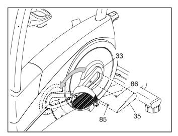
Locate the Reed Switch (57). Rotate the Left Crank Arm (20) until a Magnet (55) is aligned with the Reed Switch. Next, loosen the M5 x 16mm Flat Head Screw (60), slide the Reed Switch slightly toward or away from the Magnet, and then retighten the Flat Head Screw.
