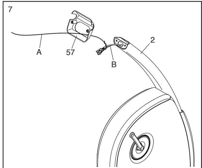
8. Orient the Handlebar (7) as shown. While a second person holds the Handlebar near the Upright (2), insert the wire tie (A) and the wires (B) upward through the Handlebar.
