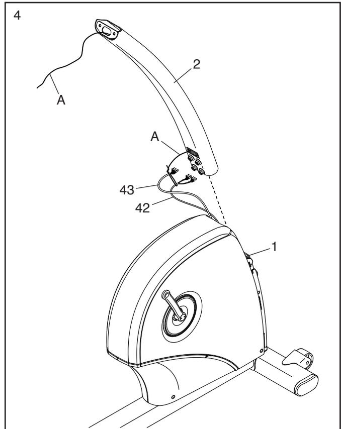
5. **Tip: Avoid pinching the wires.** Slide the Upright (2) onto the Frame (1).
