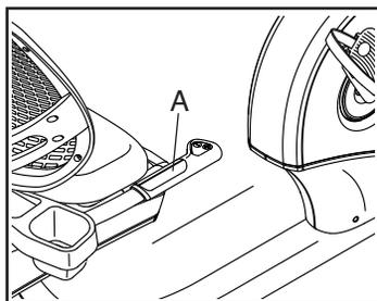
**If there are sheets of plastic on the metal contacts (A) on the handgrip heart rate monitor, remove the plastic.** To measure your heart rate, hold the handgrip heart rate monitor with your palms resting against the contacts. **Avoid moving your hands or gripping the contacts tightly.**
