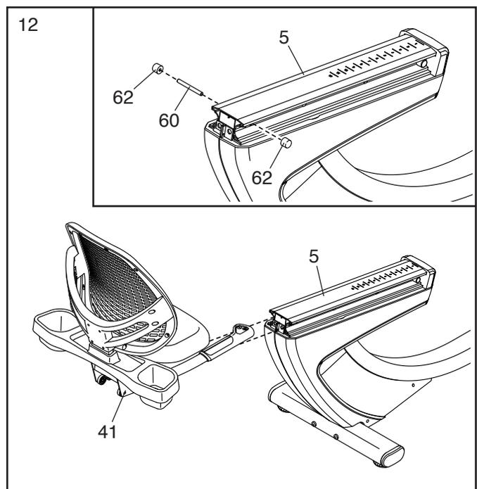
13. Insert the Rail Rod (60) into the Rail (5), and tighten a Rod Cap (62) onto each end of the Rail Rod.
